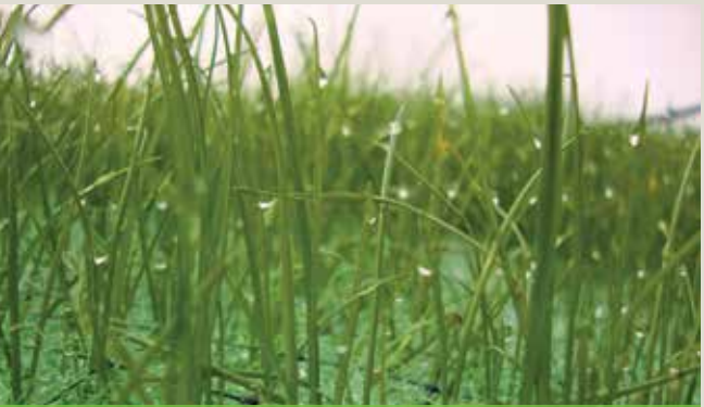
Grass seedlings growing up through synthetic Turf Reinforcement Mat (TRM) made of 100% recycled post-consumer fibers. Use to provide permanent structural root system support on vegetated slopes and in water flow channels. ©American Excelsior Company
